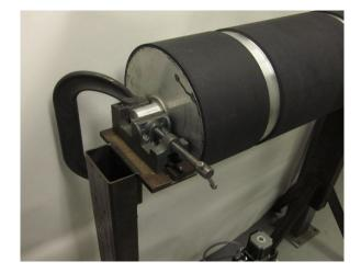
B. Clean the entire EDPM covering of the roll prior to performing the friction test. Use Efi/Vutek roll conditioner, P/N 45084568. Wait 30 minutes after cleaning process to perform Tests.
